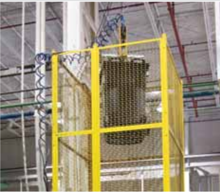
A loaded waste bin is drop tested in safety cage.
